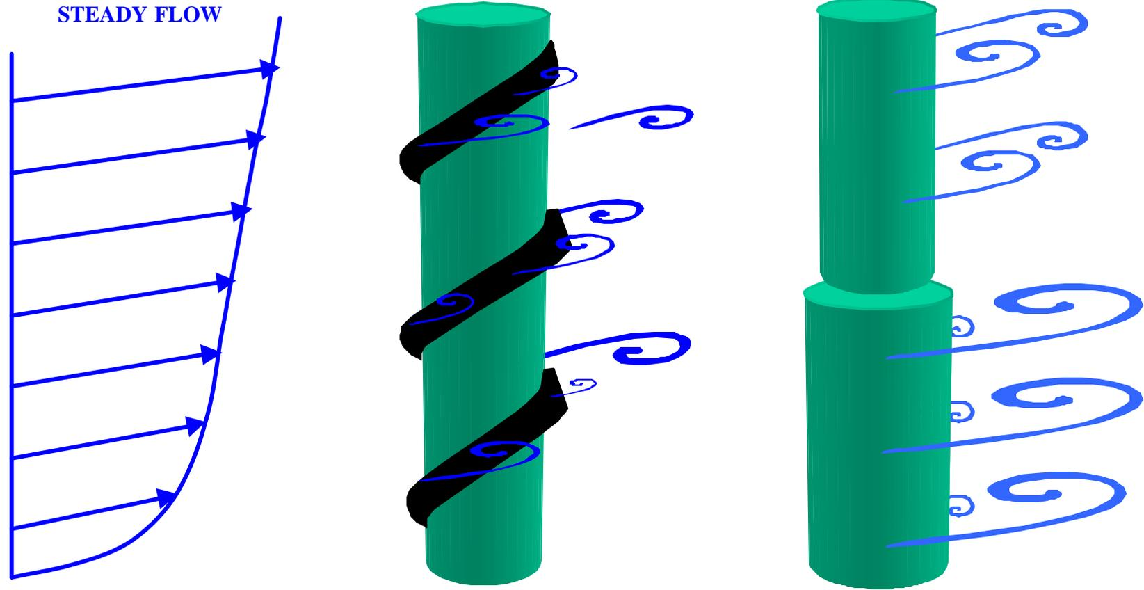
Figure 3: Vortex Shedding on a Straked Cylinder (left) and on a Cylinder with a Step-gap Discontinuity (right)
