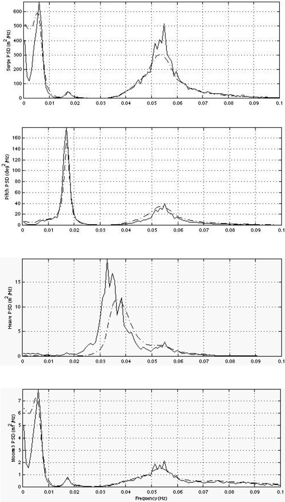
Figure 4: Comparison of Measured (solid line) and Numerically Simulated (dot-dashed line) Surge, Pitch, Heave and Mooring Tension Spectra for the 100 Year Design Storm
