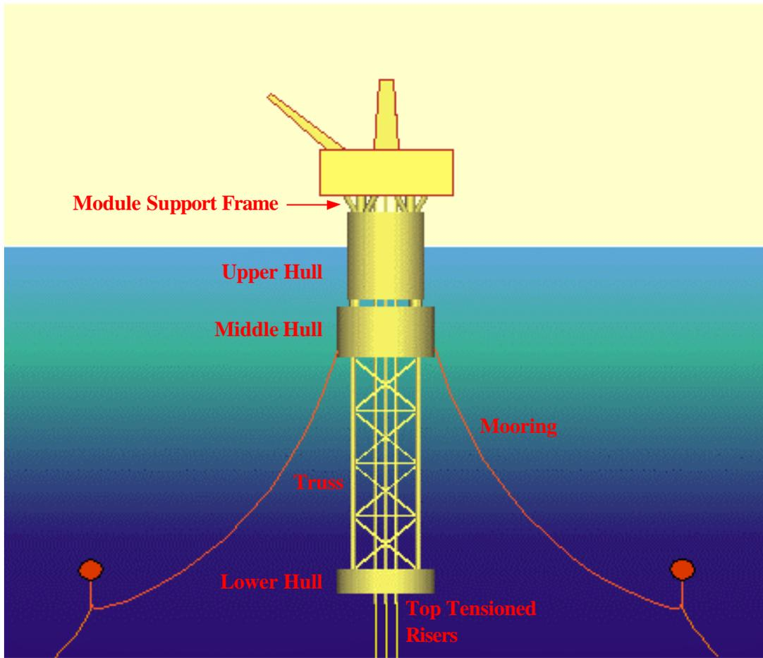
Figure 2: General Features of Hub Class Spar
